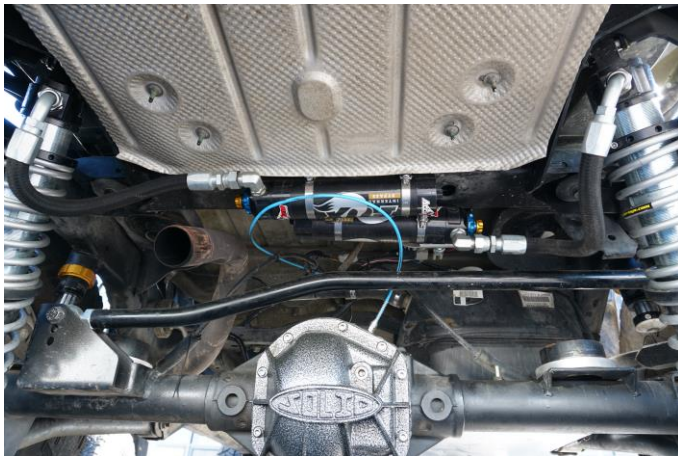
Fig 3. Front edge of mount is 1/4" away from cross member radius.
