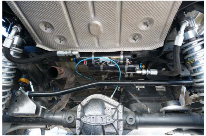
Hose Routing For Coilovers With 90 Deg Fittings
