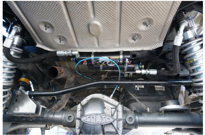
Hose Routing For Coilovers With 90 Deg Fittings
