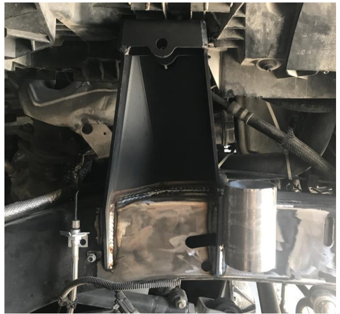
Fig 5. Frame location for upper brackets
