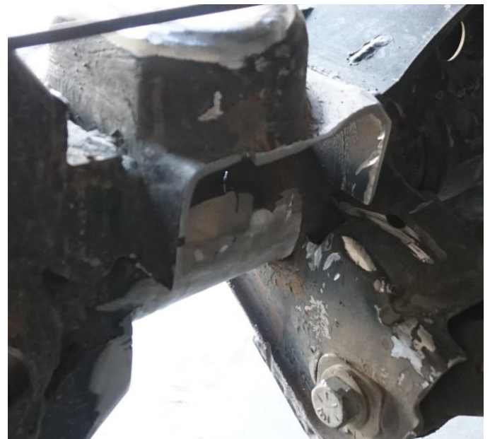
Fig 4. Where to lower shock mounts, knuckle gussets and spring perch.
