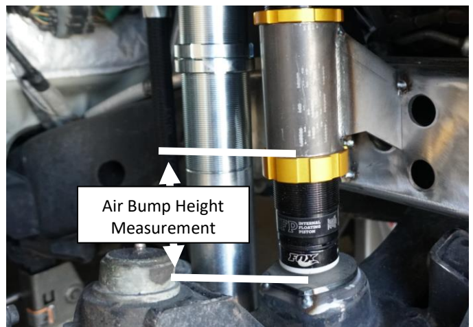
Fig 6A. Air Bump Initial Setting Measurement – OEM Fit
