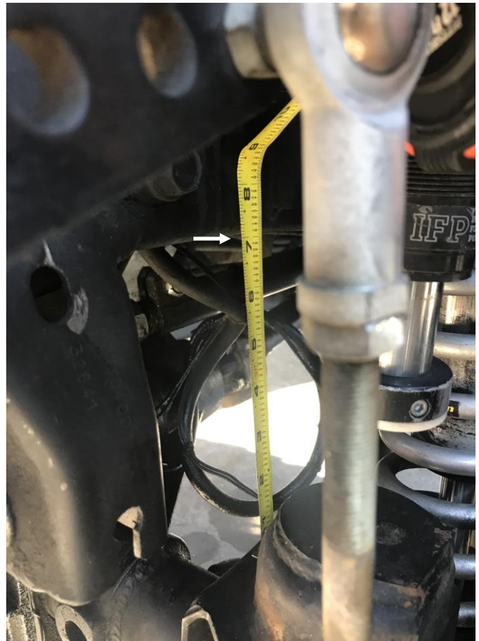
Fig 1: Front Measurement at 3" of Lift (will measure 8" for 4" lift)
