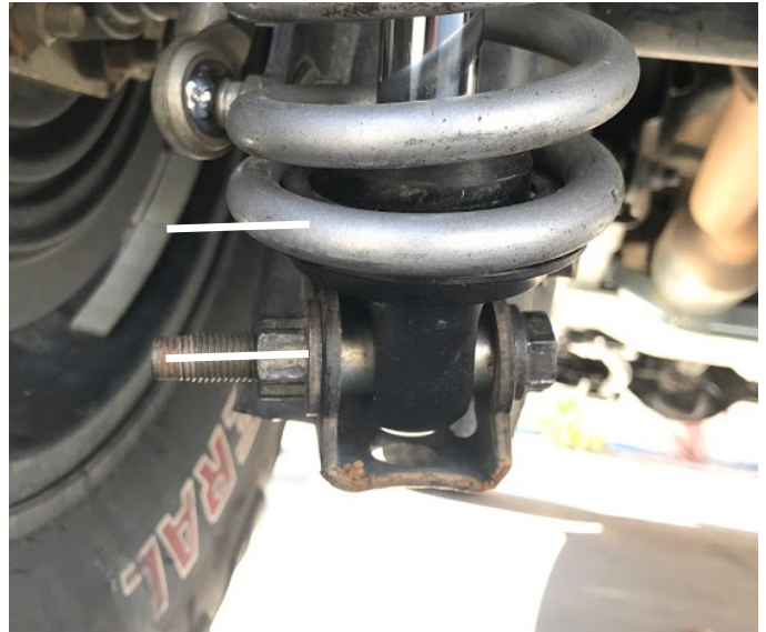
Figure 4: Reservoir bracket installation
