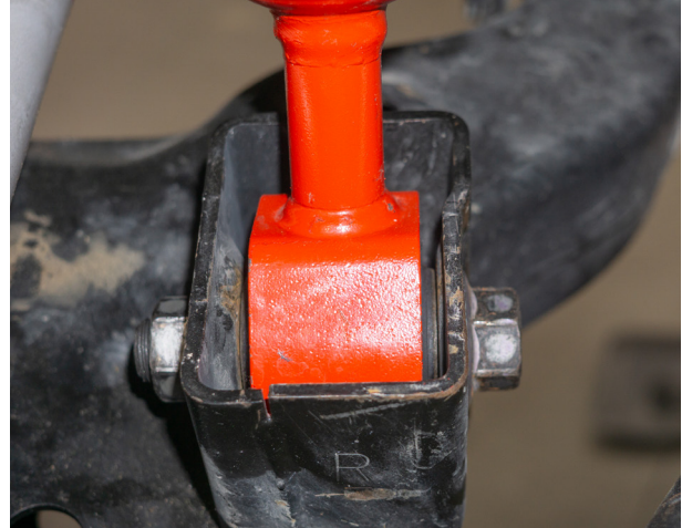
Fig. 8: Remove the bolt from the lower control arm.
