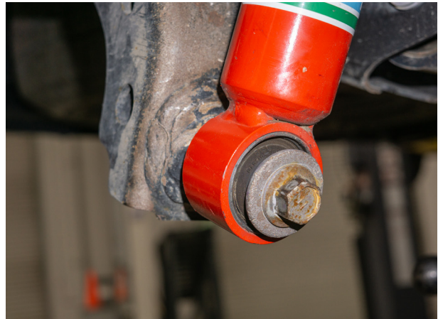
Fig. 17: Remove lower shock mount bolt.
