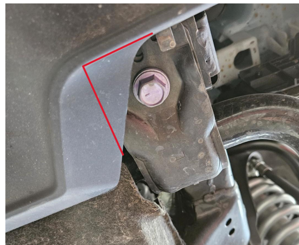
Fig. 7: Trimming area on models with front air dam.
