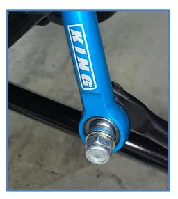
6. <u>Right Side</u> - Place the supplied 12mm bolt with washer in the sway bar link as shown below, then place the sway bar link with bolt in the mount on the frame with the longer spacer facing the mount. Place a washer and nut on the bolt and thread nut on by hand for now to hold in place, you will torque all bolts when both links are installed.
