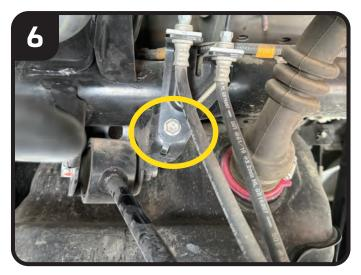
**△WARNING** 7. Slowly lower floor jack at axle, to lower the rear axle. Be sure to check for any ABS wiring or brake lines that become too tight.
