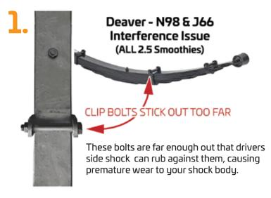
Using an angle grinder, carefully cut off the ears on the rear clip bolts. Do this before installing the leaf springs into the vehicle.
