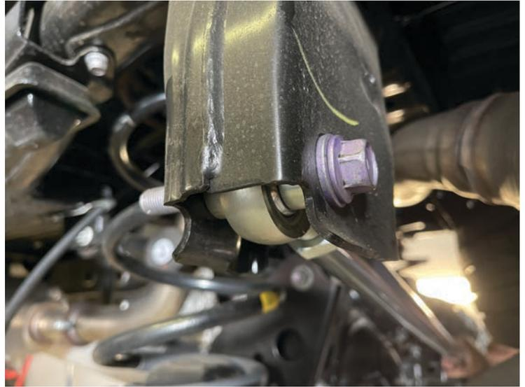
**Note:** If the holes do not line up, DO NOT adjust the heim joints! Use a ratchet strap to pull the rear end in the desired direction to line up the holes.
