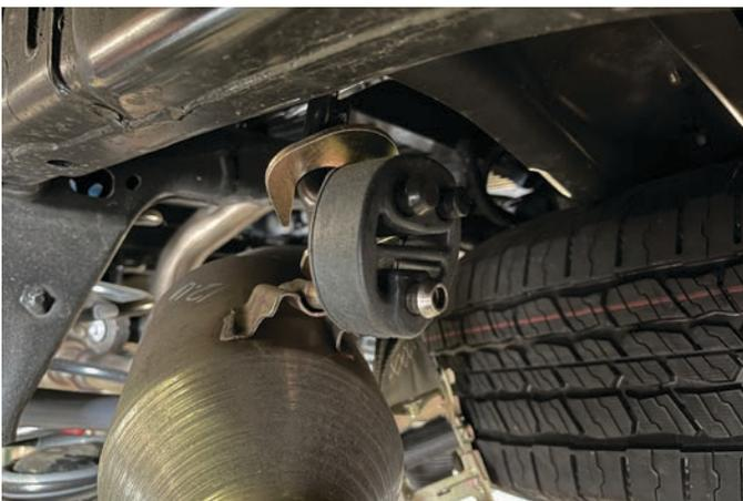
Ratchet strap shown connected to exhaust hanger.
