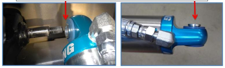
3. Install your new King Shocks with the reservoirs facing away from the axle as shown on next page. The driver's side (Left) reservoir faces towards the rear of the vehicle, the passenger side (Right) reservoir will face forward. Push the shock onto the top mounting stud with the longer spacer towards the frame and thread the factory nut on but do not tighten.
