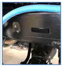
3. Insert the Backing Plate (25049-040) into the rectangular hole in frame with the rounded corners facing towards the front of vehicle. Flip the plate out with thumb as shown below and slide forward to hold in place.
