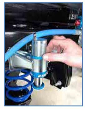
12. Make sure the set screws are backed out before tightening the upper nut. Then tighten upper stop nut using a hammer and screwdriver or punch. Tighten upper nut then tighten set screws.
