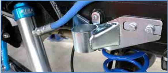
Make sure bracket is sitting flat against the side of frame and bottom of frame.
