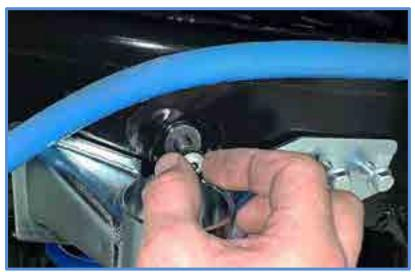
7. Use two of the factory bolts for the bottom of bracket and install into the threaded holes on underside of frame. Make sure holes are lined up and bolts are threading in easily.
