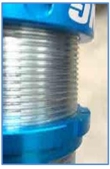
10. Thread lower stop nut all the way down as shown below.
