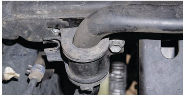
Fig. 11: Remove sway bar bracket.
