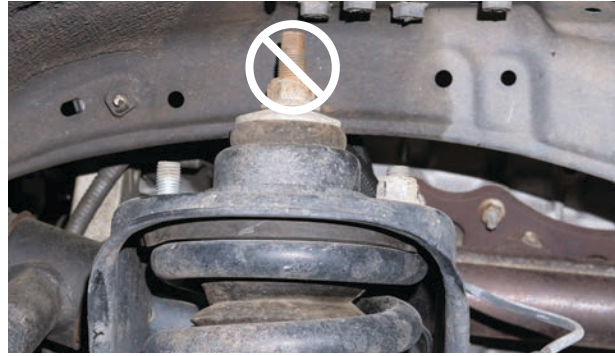
Fig. 4: Remove the three top hat nuts.
