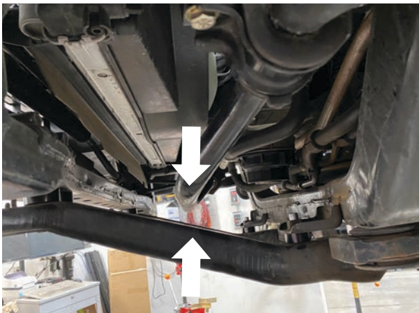
Fig. 16: Check clearance of the sway bar.
