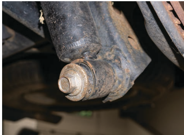
Fig. 21: Remove lower shock mount bolt.
