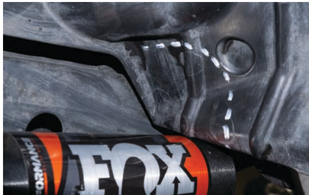
Fig. 25: Cut the fender liner.
