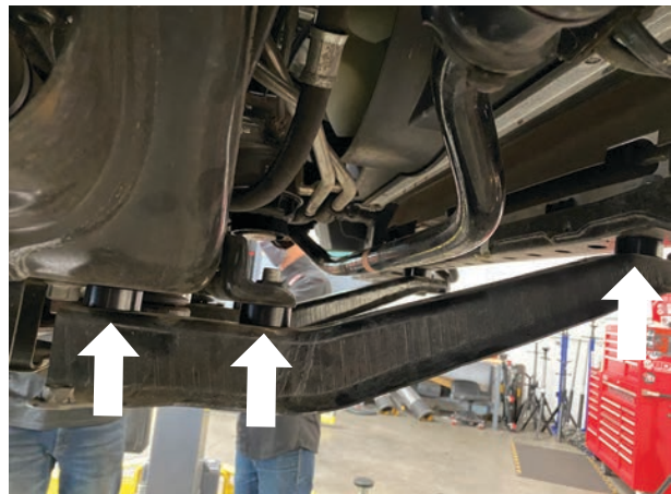
Fig. 17: Install the skid plate spacers
