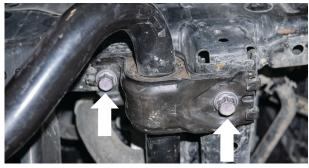
Fig. 4: Remove sway bar bracket.
