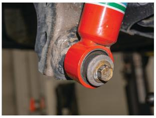
Fig. 17: Remove lower shock mount bolt.
