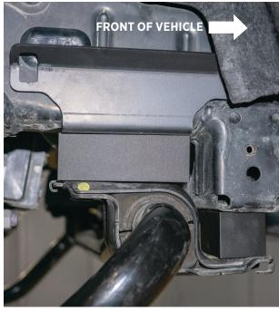
Fig. 6: Install the reservoir bracket assembly.
