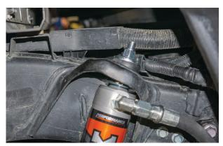
Fig. 20: Install the stem top nut (passenger side shown).
