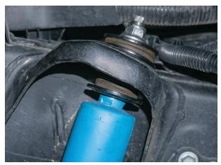
Fig. 16: Remove stem top nut.
