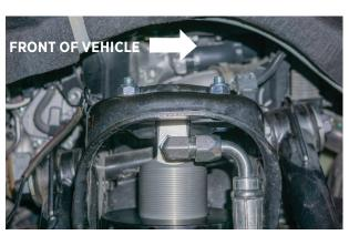
Fig. 9: The hose fitting faces outboard.
