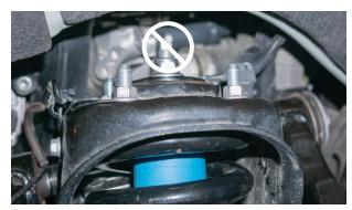
Fig. 7: Remove the four top hat nuts.
