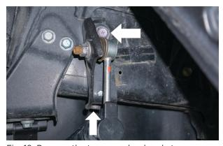
Fig. 18: Remove the two sway bar bracket bolts (passenger side shown).
