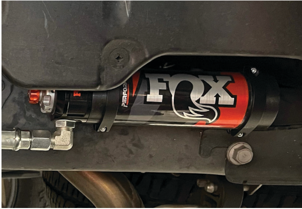
Fig 6b: Reservoir mounted to vehicle.
