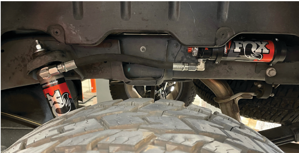
Fig 7: Installed FOX driver-side shock assembly.
