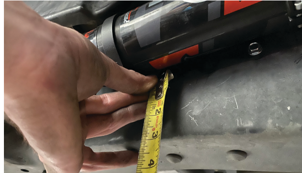
Fig 5: Measure the distance from the bottom of frame to left reservoir hole.
