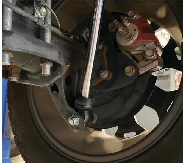
Fig 2: Install rear lower eyelet.
