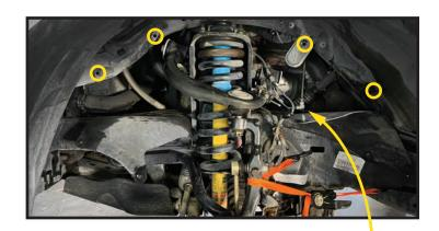
6. Unbolt the brake line bracket from frame side with a 12mm socket. This is making room for removing/replacing the upper control arm cross bolt.
