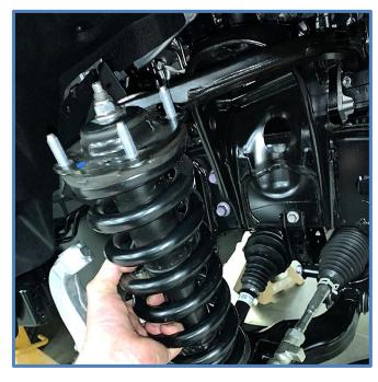
6. <u>Install King Shocks</u> – Place the rod end into the lower mount then push down on lower control arm while positioning top of shock into upper mount.
