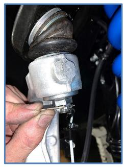
10. Reconnect tie rod and tighten nut to factory specs. Be sure to reinstall the cotter Pin.
