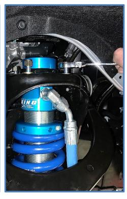
8. Insert the factory lower mounting bolt through the lower mount. Install the washer and nut, then tighten to factory specs.
