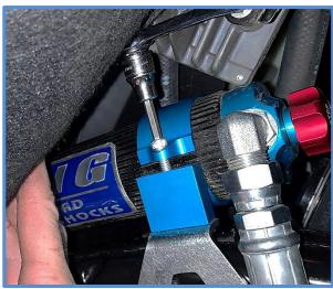
16. Lower vehicle to the ground, then install sway bar link to the lower mounting stud. Install the factory bolt and torque bolts to factory specs using a 19mm socket.
