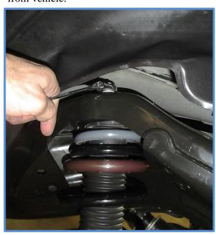
3. <u>Install King Shocks</u> – Be aware the shocks are side specific, make sure you are installing shocks on the proper side. See final install picture for reference. Place the shock into the upper mount and install the 3/8 Heavy Duty washers (CW1701) and 3/8 nuts (CN2711) on upper mounting studs and tighten nuts to hold shock in place but don't fully tighten yet.
