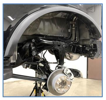
4. Place the rod end into the lower mount and install the factory bolt. Tighten lower bolt to factory specs. Torque upper 3/8 nuts to 35 ft/lbs.
