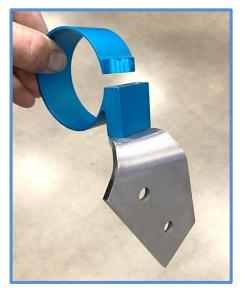
6. Slide the reservoir into the reservoir clamp, then place the bracket on the frame and line up holes in bracket with the holes in frame. Install the provided 3/8 X 1" bolts (CB4701) with HD washer (CW1701).
