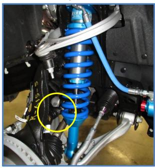
16. <u>Mounting reservoirs</u> – First attach the reservoir clamps to the reservoir brackets. Use the 1/4 X 1/2" BHCS (CB2420) to attach the reservoir clamps. Photos below show bracket for right side of vehicle. For the left side of vehicle mount clamps on opposite side of plate.
