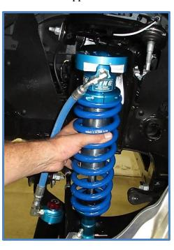
9. Install the provided 3/8" upper mounting bolts (CB4701) with HD washers (CW1701). Thread the bolts into the upper mounting plate to hold shock in place but do not tighten yet.
