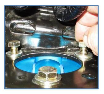
10. Install the provided 12mm X 80mm bolt (CB3829) with washer (CW1001) through the lower mounting lug and lower control arm. Place the reducer sleeve over the bolt and then install the factory nut. Thread the nut onto the bolt but do not tighten yet.
