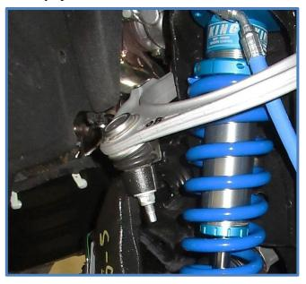
13. Now you can torque the upper and lower mounting bolts. Torque the upper bolts to 35 ft/lbs. using a 9/16 socket. Torque lower bolts to 90 ft/lbs. with an 18mm socket on the nut & 19mm wrench on the bolt head.
