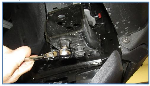
18. Slide the reservoir into the reservoir clamps then place the bracket on the front cross member and reinstall the two factory bolts.
