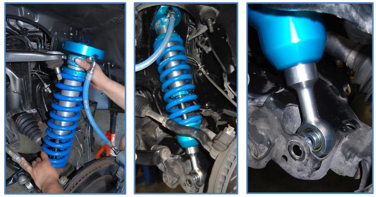
9. Line up the holes in the upper mounting plate on coilover with the upper mount on the vehicle and use the supplied 3/8 X 1" HHCS (CB4701) and 3/8 SAE HD Washers (CW1701) to attach the new coilover to the factory upper mount. Using a 9/16" socket, torque the 3/8" upper shock mount bolts to 35ft/lbs.
