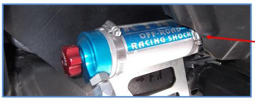
Some vehicles may require plastic trimming in the inner fender well to mount reservoir.
