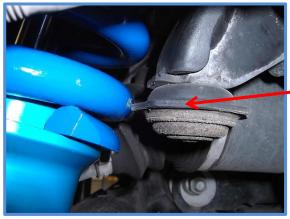
Rotate the bump stop pad or grind
