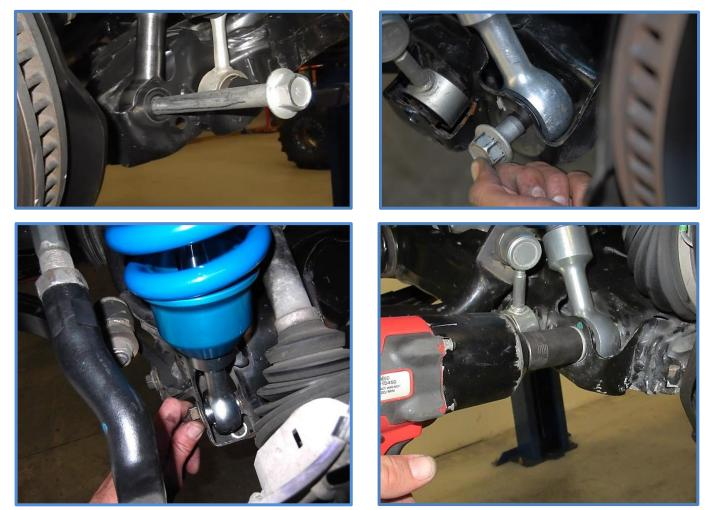
11. Check clearance at full droop, you may need to simply rotate the bump stop using a large wrench or channel locks. On some vehicles you may need to grind the bump stop bracket or HEX portion of the pad so the spring does not contact at full droop.
