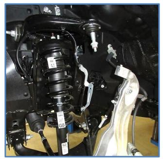
6. Complete steps 1-5 on both sides of the vehicle, then remove shocks. Remove shocks by pushing down on the lower control arm while pulling the top of shock out of the upper mount then lift the shock out of lower control arm and remove from vehicle.
