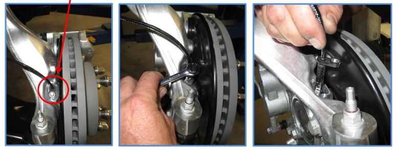
3. Remove the upper mounting nuts using a 15mm wrench or socket.
