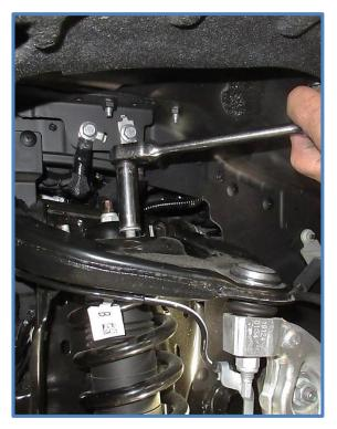
4. Remove the lower mounting nuts using an 18mm wrench or socket.
