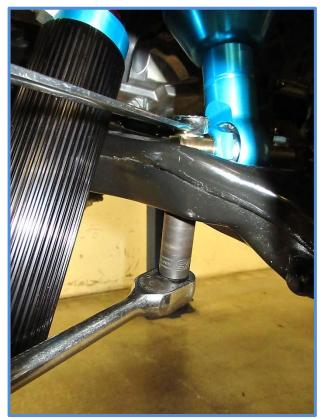
12. Install the ABS sensor, ABS bracket and brake line bracket.
