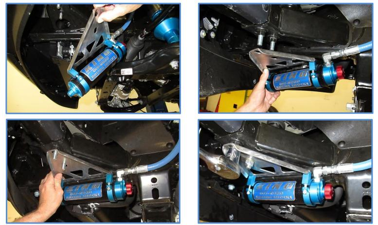
16. Install the 1/4 X 1" bolts (CB1501) in the reservoir clamps and tighten using a 3/16 Allen wrench.
