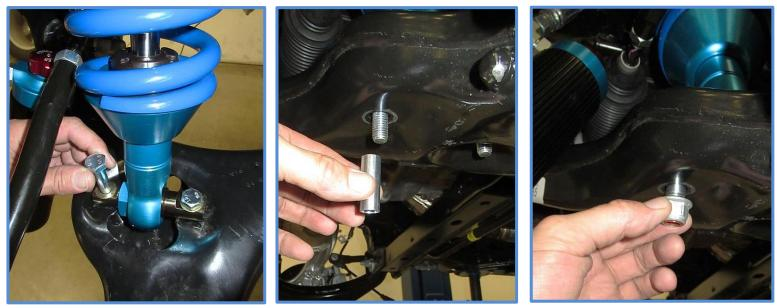
10. Reconnect the upper control arm and tighten nut to factory specs. You may need to hold the stud with an 8mm wrench as shown below to keep the ball joint from spinning while tightening nut.
