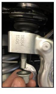
5. The only thing holding the stock upper control arm on the car is the through bolt, slide the through bolt rearward out of the stock arm and remove the arm.
