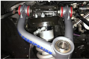
10. It is now time to rotate the UCA down and connect it to the spindle using the supplied tapered adapter and supplied hardware. Slide the 14mm 2.0 socket head bolt through the upper misalignment, lower misalignment, tapered adapter, spindle, washer, and into the supplied 14mm 2.0 flange nylock nut. Tighten the bolt using a 12mm Allen wrench
