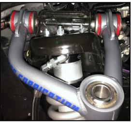
9. Once the arm is installed put the new nylock nut onto the through bolt and use a 21mm wrench and 18mm wrench to tighten the through bolt (101 ft/lb).
