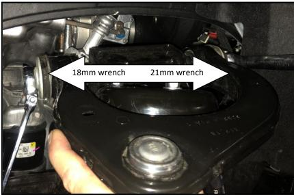
4. Remove the stock upper ball joint nut and carefully lift the arm out of the spindle making sure the spindle doesn't lean too far outward and dislodge the inner CV joint.
