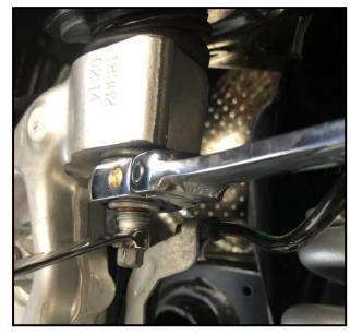
3. Using an 18mm and 21mm wrench, loosen the upper control arm through bolt and remove the nut. The passenger side has a heat shield that covers the rear control arm pivot, this heat shield needs to be removed using an 8mm wrench. The shield will be reinstalled after the new Total Chaos UCA's are installed.
