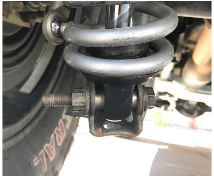
Figure 3: Lower coilover spacer installation
