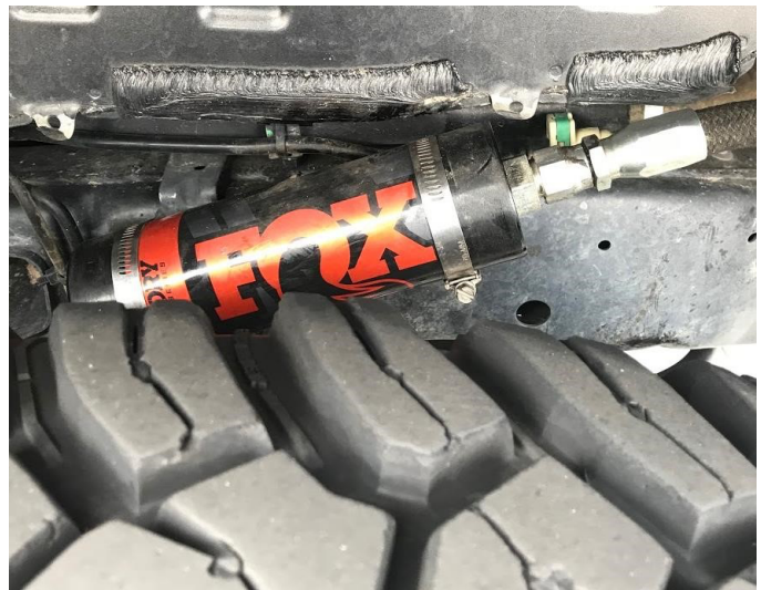
Figure 4: Reservoir bracket installation
