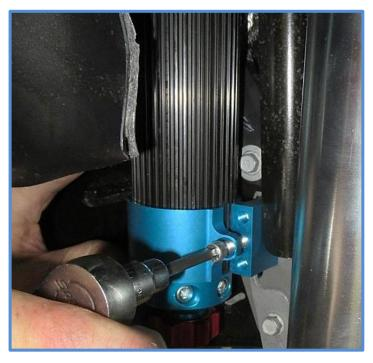
11. Place the rod end into the lower mount, install the factory bolt and tighten to 60 ft-lbs.
