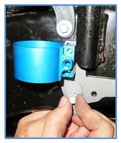
7. Now use the bent threaded nut plate included in the kit to secure the reservoir bracket on the other end. Place the nut plate in the large hole in the frame and line up with the hole in the reservoir bracket. Use the 1/4 X 1" bolts (CB4502 with washer CW1501) to thread into the nut plate.
