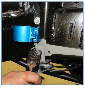
9. <u>Installing Shocks</u> – Be aware the shocks are side specific, make sure you have the proper shock for the side you are working on. Begin placing the shock into position on the vehicle while inserting the reservoir into the clamp. Place the end cap into the upper mount, install the factory bolt and tighten to 60 ft-lbs.
