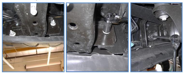
11. With the bumper removed you can now access the tow hook holes in the frame. Position the reservoir mount on the frame (as shown in the photos below) and install using the supplied 10mm hardware.
