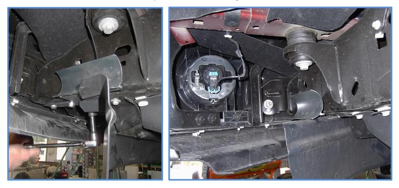
13. Install King Remote Reservoir Shocks by first feeding the reservoir through the hole at the top of the shock mount. Be aware that the shocks are side specific, the reservoir will route towards the front of vehicle as shown in the photos below.
