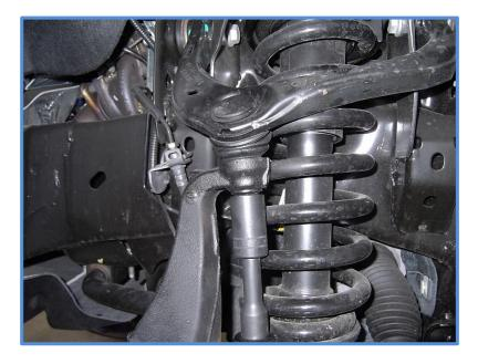
5. Using a 15mm socket, remove the three nuts from the top of the shock assembly and remove the shock.
