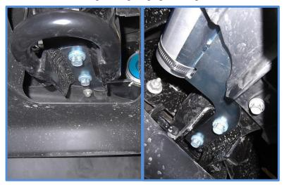
8. Open the hood to access the hood latch bolt and two other bolts that need to be removed. Use a 10mm socket for the hood latch bolt and an 8mm socket for the other two bolts. Also, make sure the hood latch cable is unclipped from the fascia.
