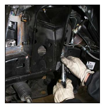
(After install is complete) (Shocks installed) Adjust the limit straps so that there is a ¼" gap between the high mis-alignment space and the uni-ball cup on the upper control arm. (Take measurement at full droop) Limit straps will stretch over time and will need to be adjusted periodically to prevent damage to the shock and uni-ball components.
