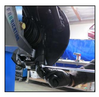
Step 16: (Tie-rod extension install) Remove the stock outer tie-rod end from the inner tie-rod. Install tie-rod extension provided onto outer tie-rod using anti-seize and tighten all the way. Thread onto the inner tie-rod (Do not tighten at this time, An alignment will need to be done.) Place ball joint end into spindle and secure with the factory castle nut. (Torque nut to 75ft/lbs 101-NM and install new cotter pin.)
