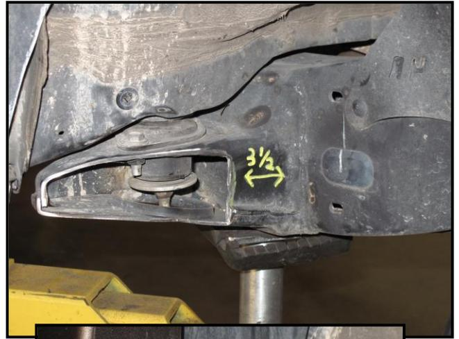
3. The inner fender well, as well as the fender flare will need to be trimmed using a disk cutter and box cutter to optimize tire clearance.
