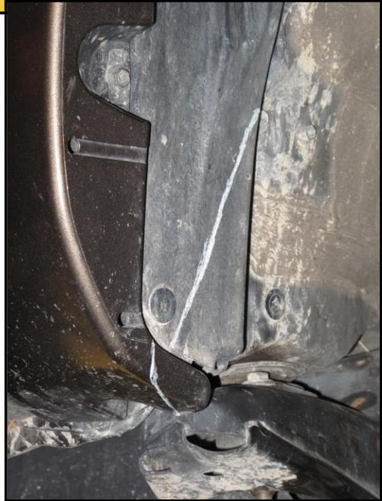
4. Once the sketch line is on the body mount cut along the line (make the cut slightly smaller than the line, you can always cut more off, if the plate doesn't fit).
