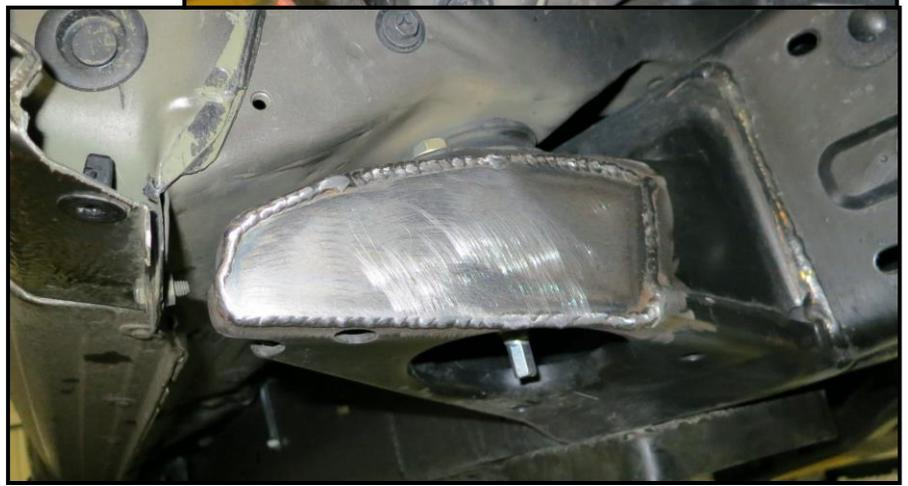
get it to fit perfectly. Once it is fit, tack it in place and turn your tires back and forth to make sure the clearance is sufficient. If so, weld the new plate to the body mount.
