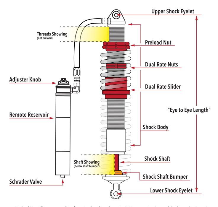
**Preload Nut:** Allows you to adjust the preload on the coilover shock. For zero preload, extend shock completely and have the proload nut resting against the upper spring not allowing the springs to move up or down.
